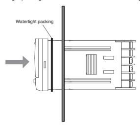
(3) Insert the adapter into the grooves on the left and right sides of the rear case and push until it reaches the panel and is fixed in place.
