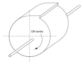
As shown in the above diagram, when rotating a cylindrical object and measuring the distance from the object using a laser displacement meter, it cannot be judged if the increase in measurement values when the rotating axis is eccentric is due to the eccentricity or to a burr.
