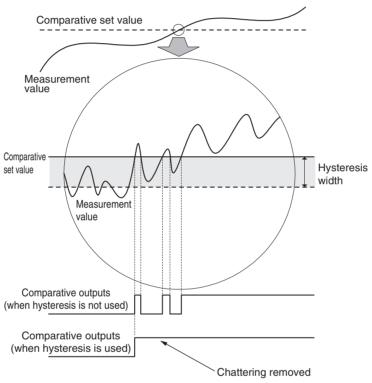
Hysteresis works in direction of decreasing measurement values for comparative set values HH and H and works in the increasing measurement value direction for comparative set values LL and L.
