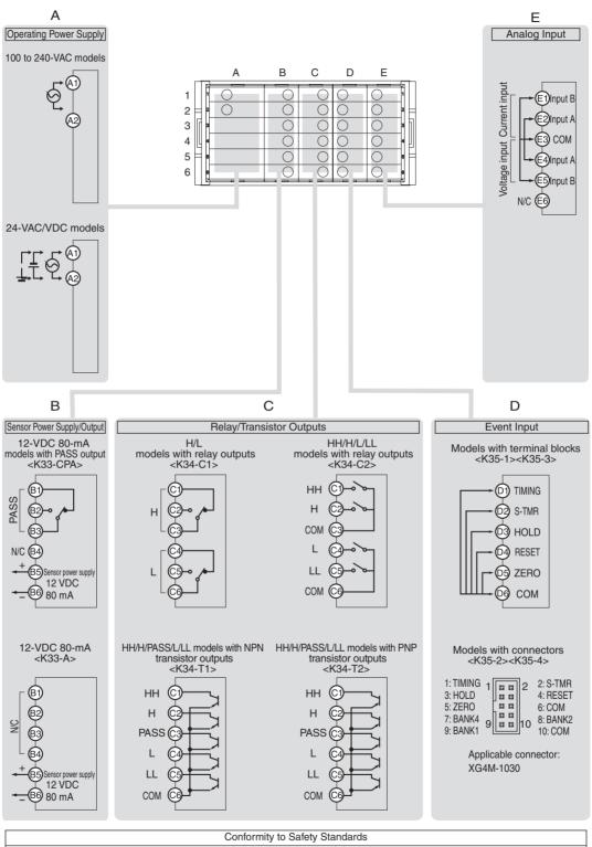
The device uses reinforced insulation between the power supply, the inputs/transistor outputs, and the relay outputs, however, basic insulation is used between the inputs and the transistor outputs.
