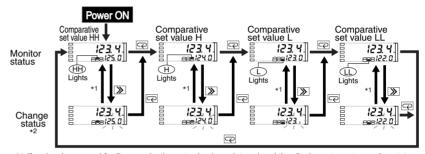
\*1 If no key is pressed for 5 seconds, the set value is registered and the display returns to monitor status.
