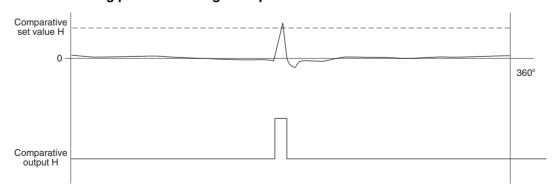
Previous average comparison makes the measurement value the difference between the present input value and the average of all previous input values.
