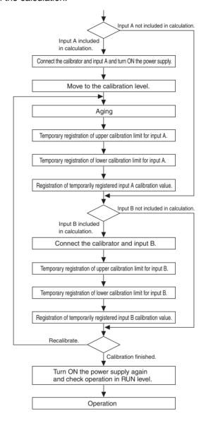
The input type that can be calibrated according to this flowchart is the type selected under "input type A" or "input type B".
