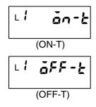
TIMING inputs can be delayed by adjusting the ON timing delay and OFF timing delay.
