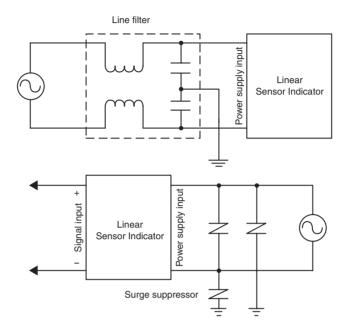
(2) In order to prevent inductive noise, wire the lines connected to the terminal block separately from power lines carrying high voltages or currents. Do not wire in parallel with or in the same cable as power lines. Other measures for reducing noise include running lines along separate ducts and using shield lines.
