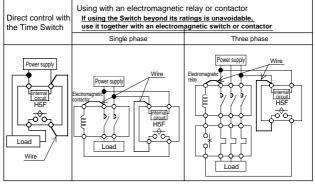
Applicable wire : 600V vinyl-insulated wire (solid wire or stranded wire, copper) 14 to 24 AWG
